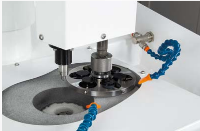
Prepolishing of coated samples, mounted on a central pressure sample holder.
