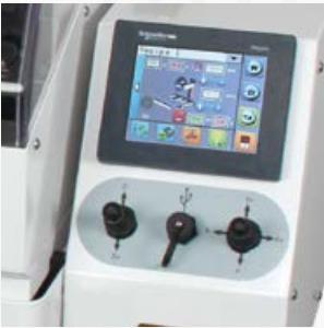
Quick positioning with joysticks. Touch screen with graphical interface.
