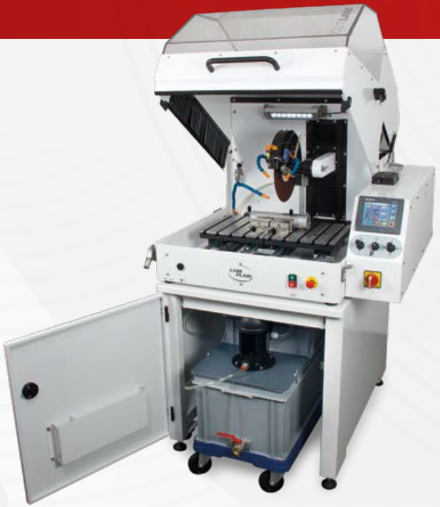
Support cabinet with integrated cooling system (60 litres).
