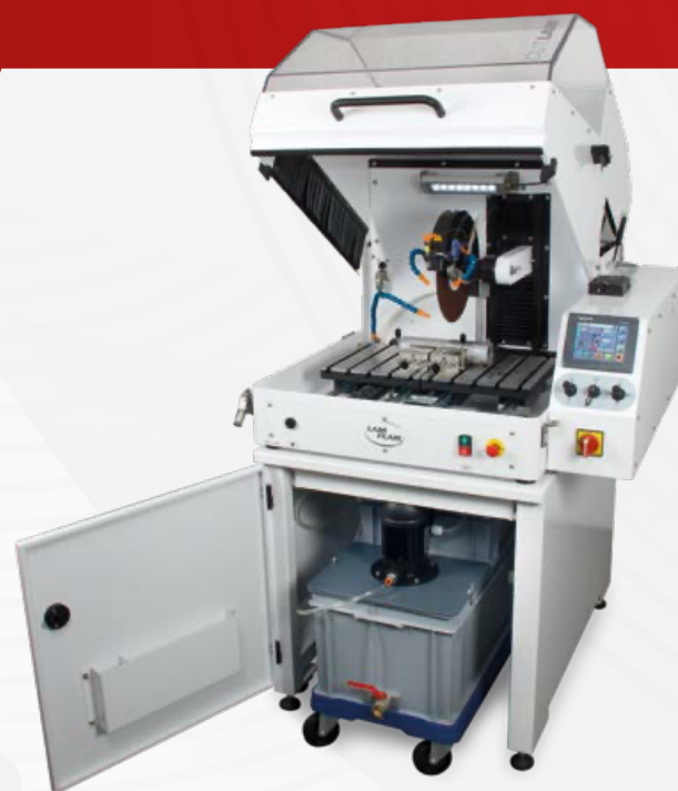
Support cabinet with integrated cooling system (60 litres).
