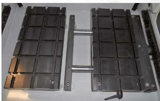
Transversal table X axis 120 mm stroke
