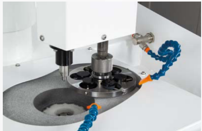
Prepolishing of coated samples, mounted on a central pressure sample holder.
