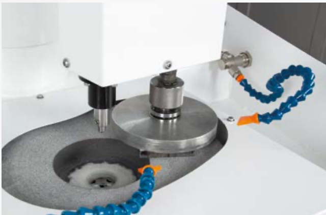
Prepolishing of large raw samples.
