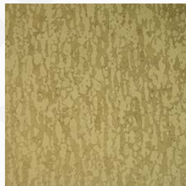
TA6V titanium etched by Kroll reagent
