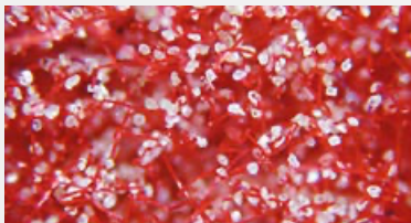
Flocked viscose fibres
