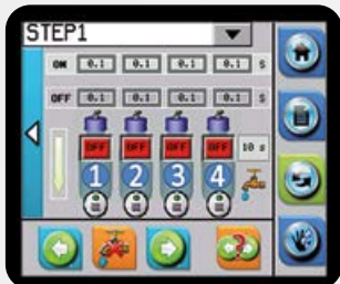
DISTRILAM dosing unit programming integrated to the machine's commands in the full range of MASTERLAM® machines.
