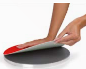
Self-adhesive cloth on FAS® 2 support
