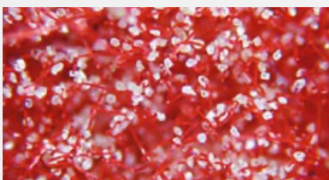
Flocked viscose fibres
