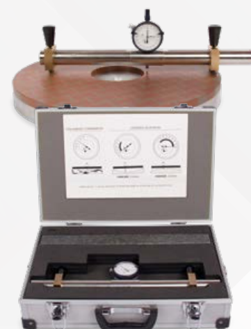
Micrometric gauge for Ø 200 to 600 mm machines
