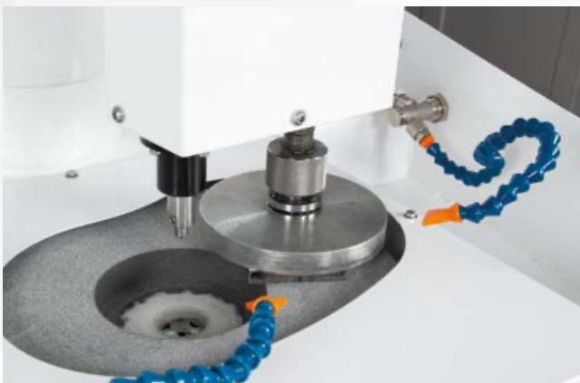
Prepolishing of large raw samples.
