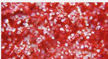
Flocked viscose fibres
