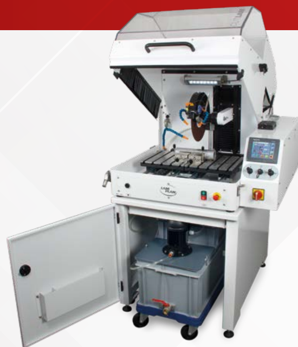
Support cabinet with integrated cooling system (60 litres).
