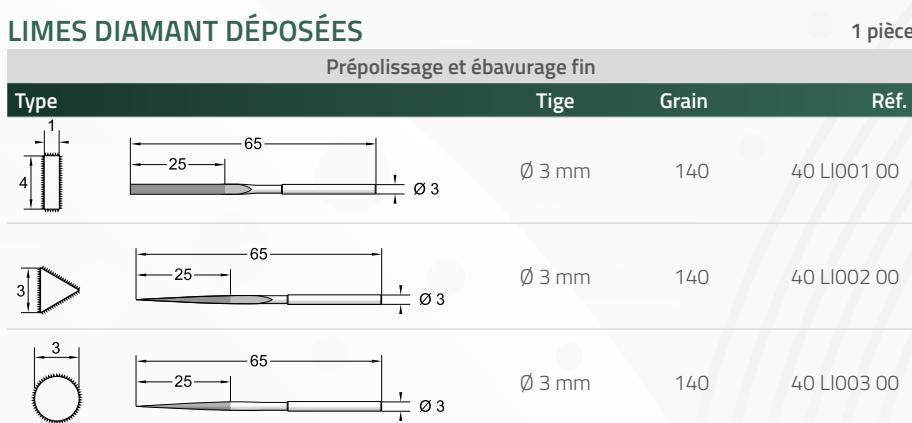
Diagram showing three types of diamond files for grinders with their dimensions and a table of file sizes with their corresponding dimensions and references.
