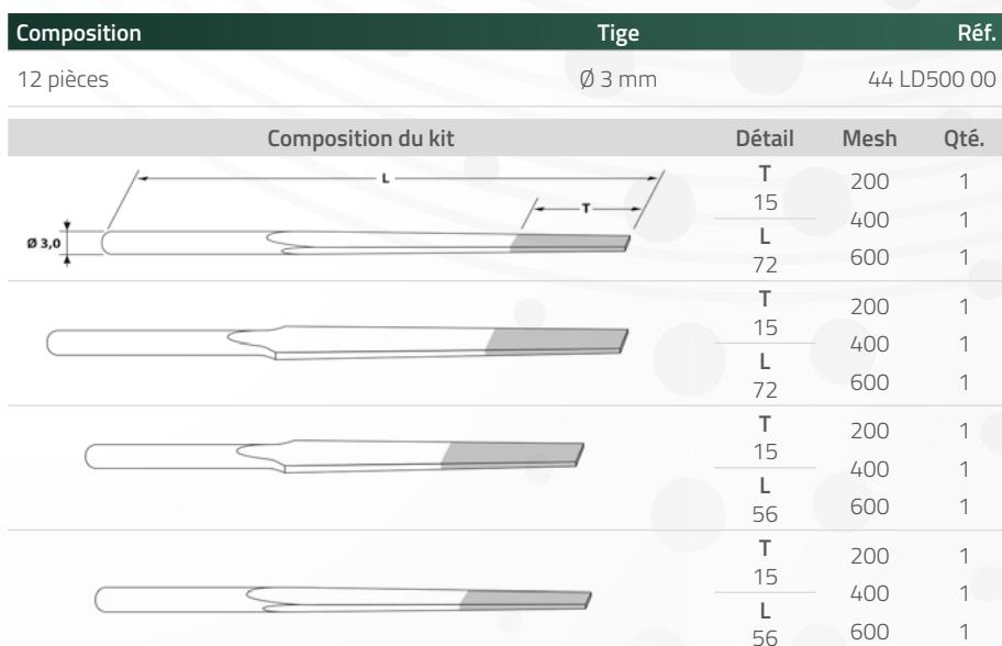
Diagram showing a diamond file kit with four types of files and a table of kit contents with their corresponding dimensions and quantities.
