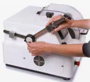
Manual micrometric adjustment of the Z axis.
