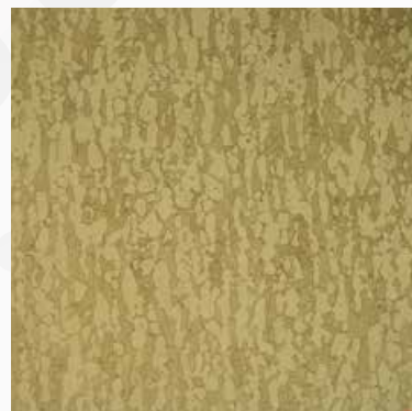
TA6V titanium etched by Kroll reagent
