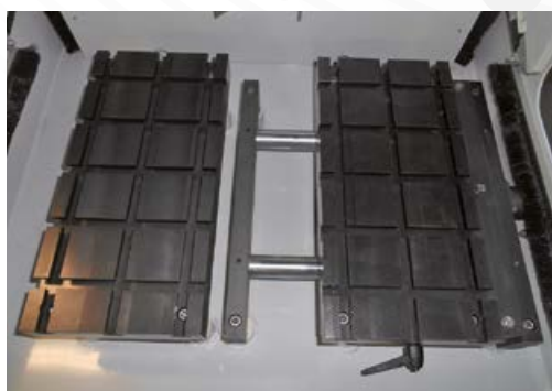
Transversal table X axis 120 mm stroke
