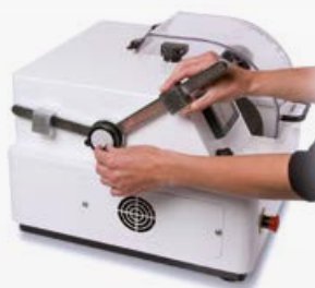
Manual micrometric adjustment of the Z axis.
